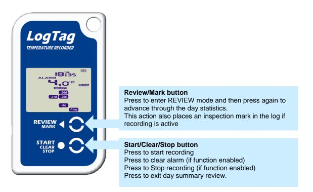
Start/Stop/Clear button functions require the button to be pressed continuously for 4 seconds and then released when the related flashing indicator stops flashing. This reduces the possibility of vibration or a load being placed on the recorder that causes permanent or intermittent button press to falsely trigger a function.
